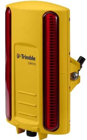
**Linear Detection** – Exact laser strike positions to within 1.5mm (0.06") for precise automatic grade control. Unlike other laser receivers that provide only 5 to 7 fixed relative grade regions, the LR410 provides a continuous, absolute laser strike position to precisely measure the actual height deviation from “On Grade.” This feature gives you the highest accuracy and grade performance.
