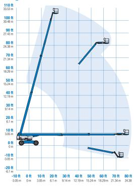
$<sup>^{\</sup>star}$  The metric equivalent of working height adds 2 m to platform height. U.S. adds 6 ft to platform height.
